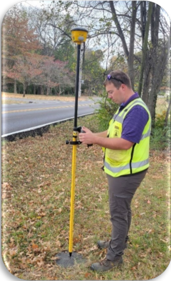
Figure 7- Construction Coordinator II Tyler Phelps conducts survey work along Highland Way. He dropped over 2,300 points for sidewalk planning between Nashville Road and Smallhouse Road (5 November)
