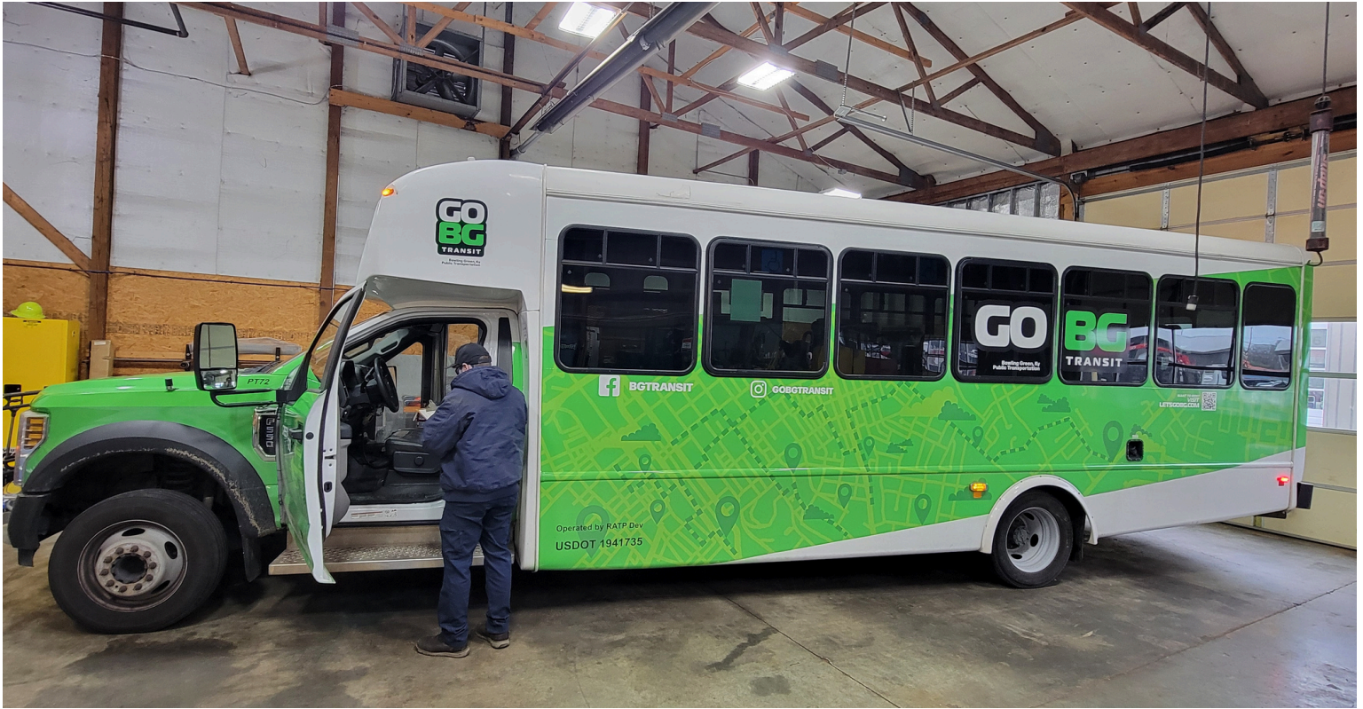
Service Technician Nick Updegraff performs a safety inspection on a Go BG Transit Bus (13 February).
