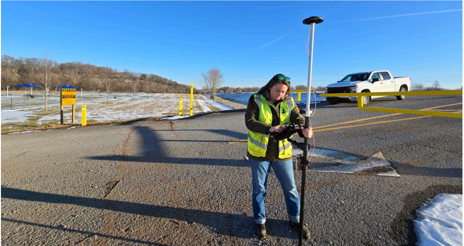
Environmental Compliance Inspector Courtenay Howell collects data points of high water marks with the divisons new Global Navigation Satellite System device at Phil Moore Park (21 February)
