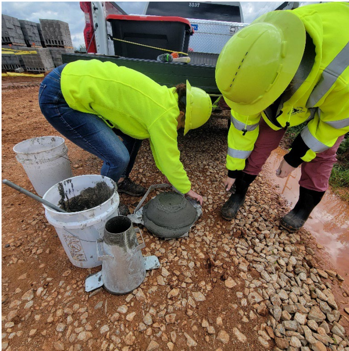
Figure 7- Construction Coordinator II Melanie Shy (Left) and Construction Coordinator I Dara Price (Right) conduct mortar testing at the new Public Safety Training Complex site on Porter Pike. Mortar is tested for strength and slump. (3 April)
