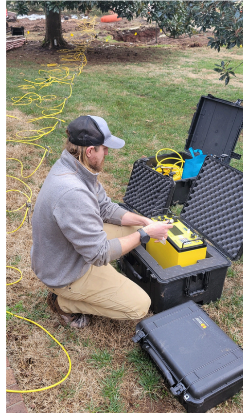
Above - City Geologist Nick Lawhon assesses a sinkhole on Single Tree Way utilizing electrical resistivity tomography (13 January).
