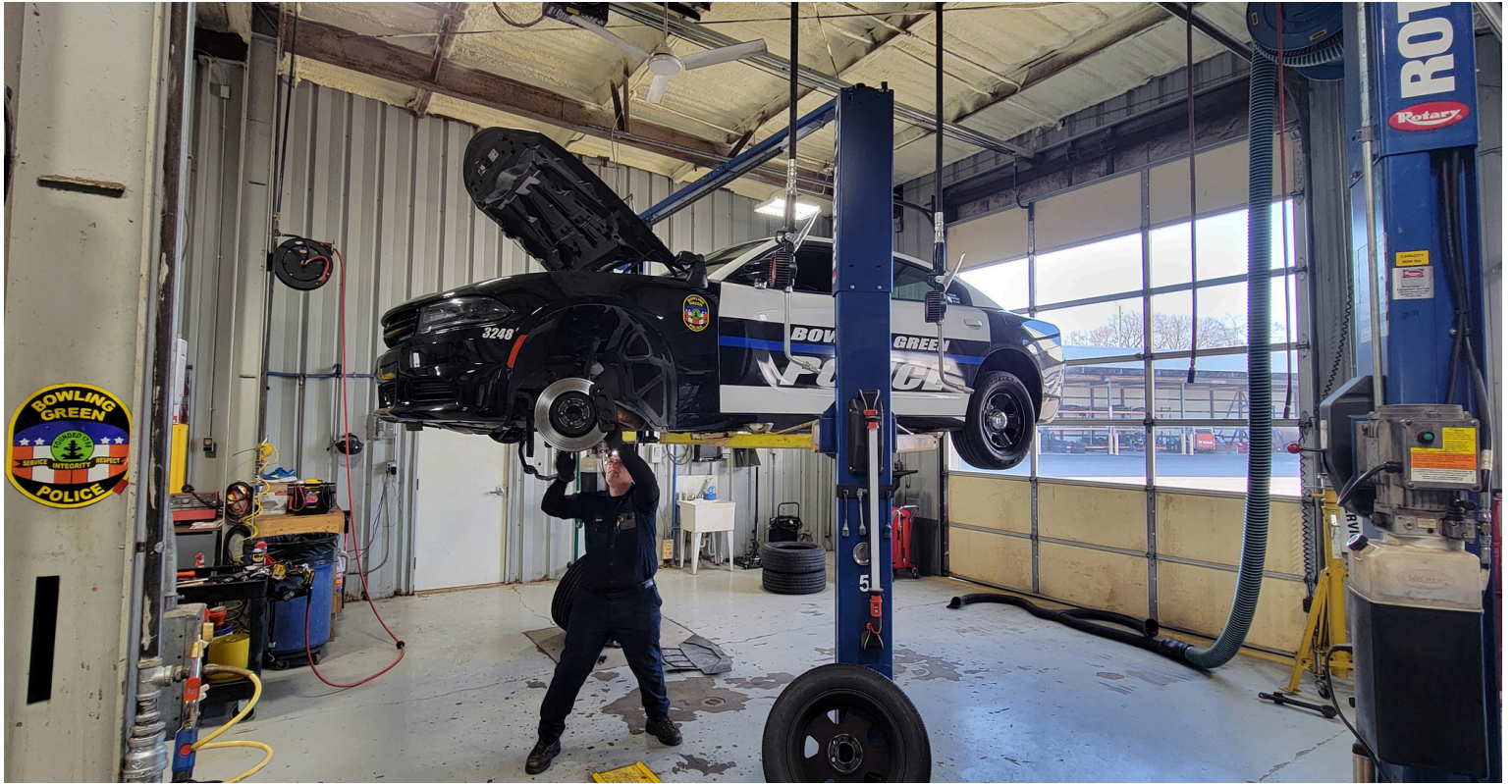
Service Technician David Long replaces the brakes on a BGPD cruiser (27 January).
