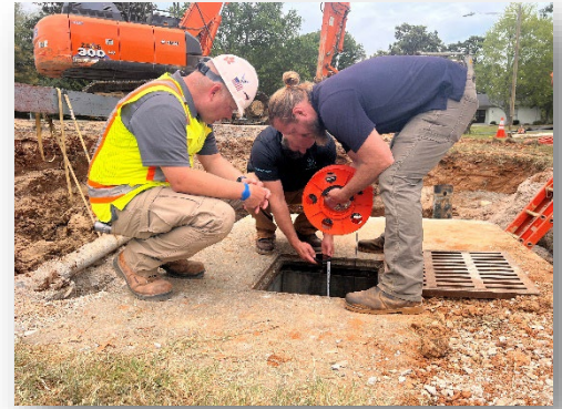
Figure 7- Director Andy Souza, Environmental Manager Matt Powell and City Geologist Nick Lawhon assess the depth and functionality of a 1970's era injection well located at the Single Tree Way sinkhole site (12 Sep)
