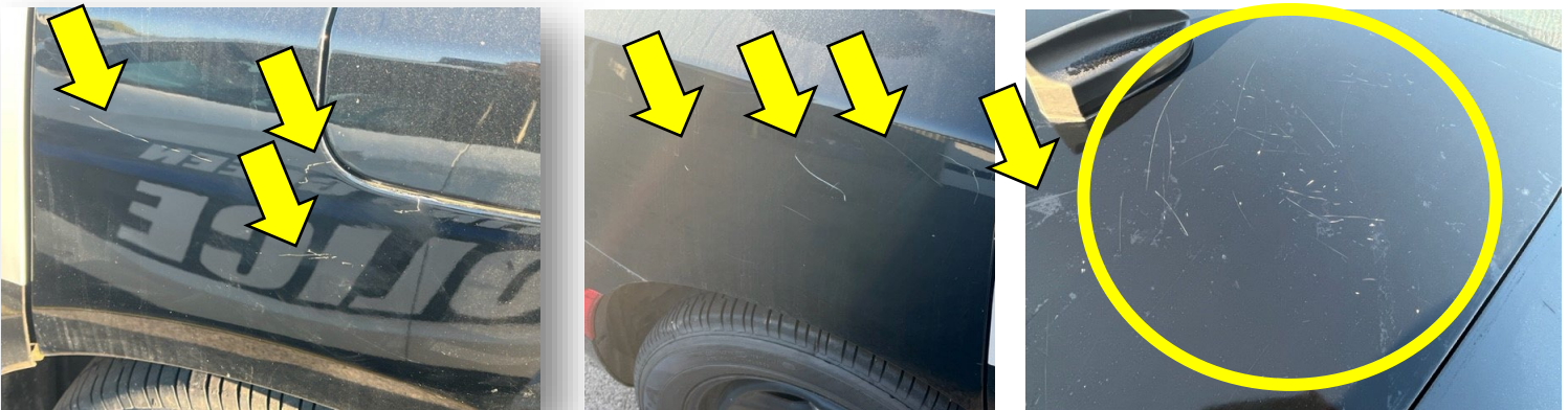
Figure 12- Unit 3229 (2016 Dodge Charger Police RWD) required quarter panel, trunk lid and rear lamp work. This is an example of the daily wear and tear on city vehicles. Repair cost was $1,846 (12 September)
